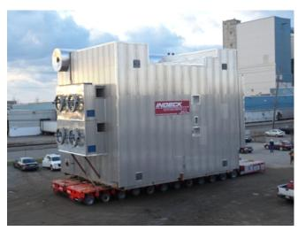
Erie, PA... Indeck Keystone Energy's technology center has completed the custom engineering and manufacture of one of the largest shop-assembled boilers in the United States. Indeck Keystone Energy delivered this massive Keystone watertube "D" type package boiler for a major steel manufacturer in the Midwest. The boiler weighed nearly 1,000,000 pounds and required tremendous efforts to move it by land and sea to the client.
