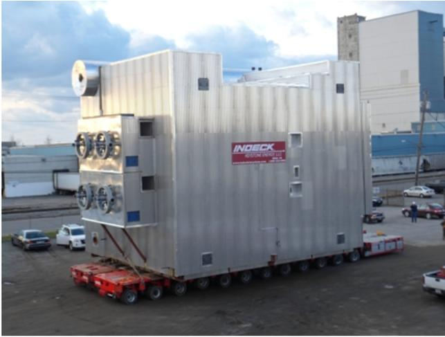
Erie, PA... Indeck Keystone Energy's technology center has completed the custom engineering and manufacture of one of the largest shop-assembled boilers in the United States. Indeck Keystone Energy delivered this massive Keystone watertube "D" type package boiler for a major steel manufacturer in the Midwest. The boiler weighed nearly 1,000,000 pounds and required tremendous efforts to move it by land and sea to the client.
