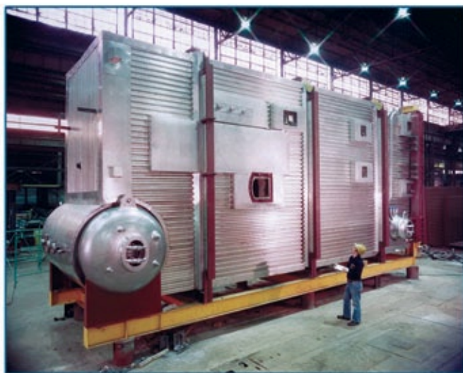
• Shop Assembled 2-Drum Boiler ready to ship •
